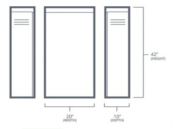
The NeoVolta NV24 is an additional battery capacity option. When combined with the NV14, total energy storage capacity is increased from 14.4 kWh to 24.0 kWh of Lithium Iron Phosphate (LiFePO4) rechargeable battery.
